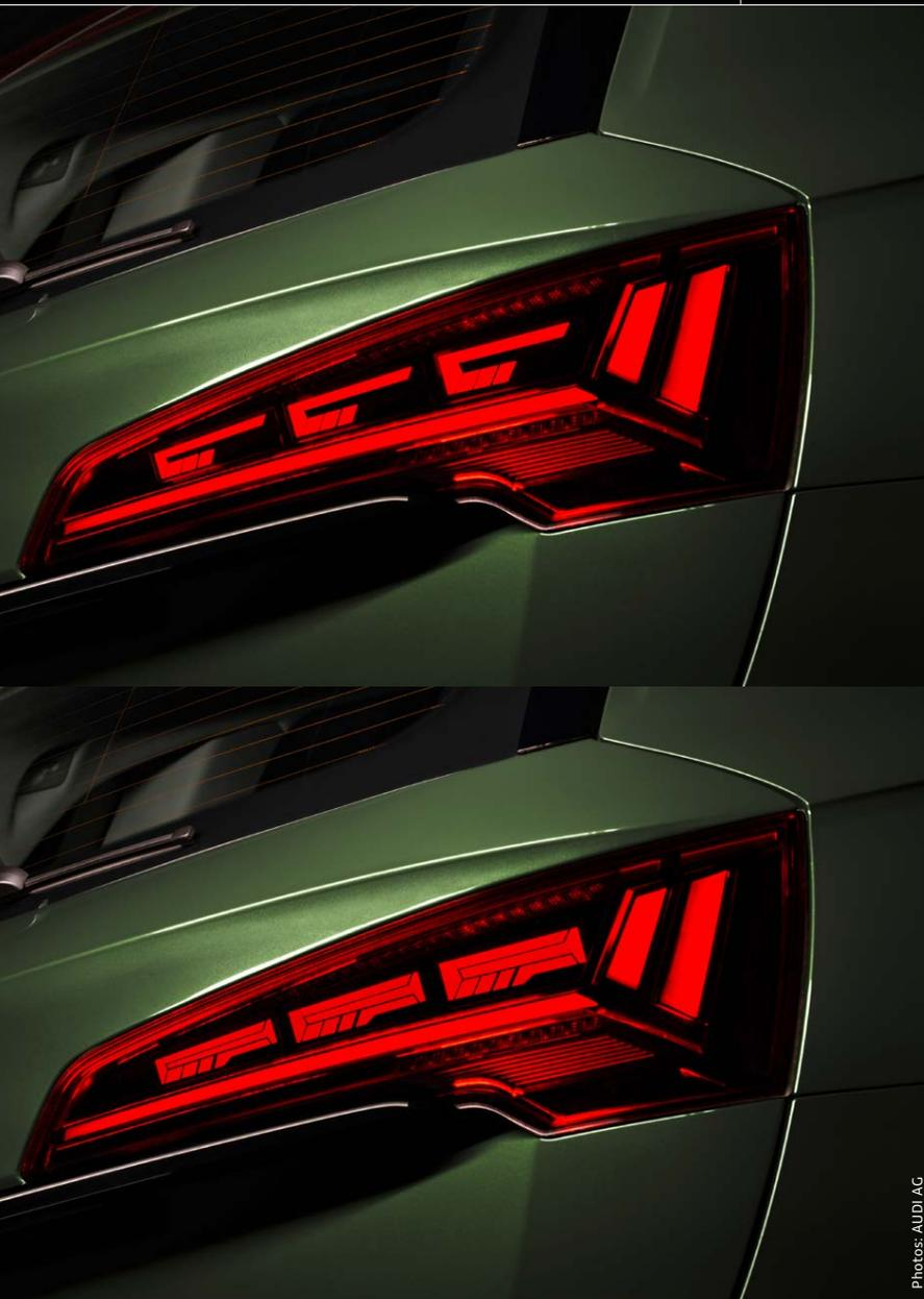
An Audi Q5 rear light has three panels, each incorporating six OLED segments. These can now be activated as needed, and their brightness adjusted infinitely. The optional proximity detection by activation of all OLED segments can be seen at the bottom.
