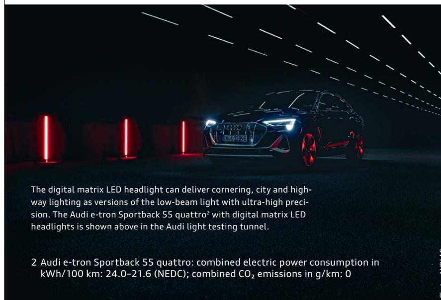
The digital matrix LED headlight can deliver cornering, city and highway lighting as versions of the low-beam light with ultra-high precision. The Audi e-tron Sportback 55 quattro<sup>2</sup> with digital matrix LED headlights is shown above in the Audi light testing tunnel.
